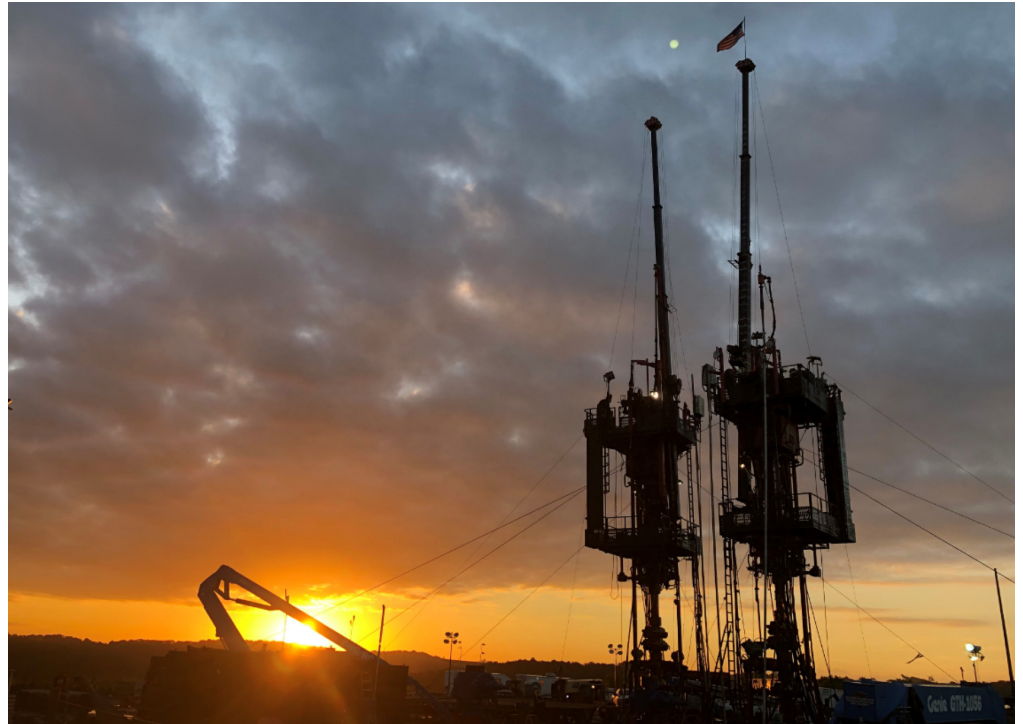
Figure 1: Hydraulic Completion Units (HCUs)
